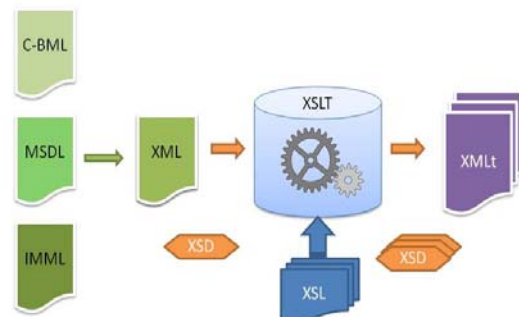
Figure 4. CSES Data Exchange Mechanism logical architecture
