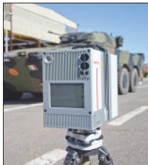
Figure 1: 3D Terrestrial laser scanner at NATO M&S COE
