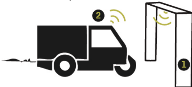
Picture 2: Scheme representative portal for capturing identification signals. Part of the localization system. 1 - Portal with antennas / 2 - Truck tagged RTLS
