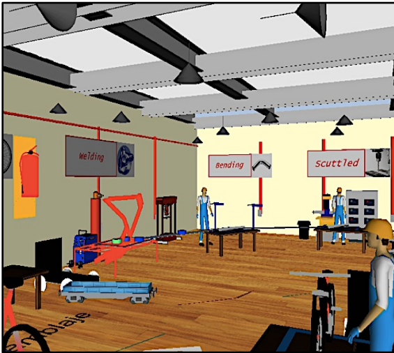
Figure 7: The simulation model of the manufacturing process of e-bikes: the welding, bending and scuttled processes
