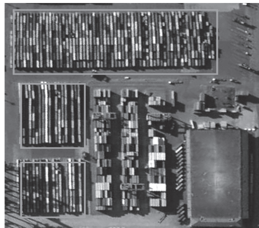
Figure 4. Inventory of the maritime port depositories based on the remote sensing data treatment
