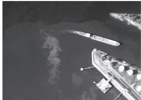
Figure 3. Remote sensing identification of the ship bilge water
