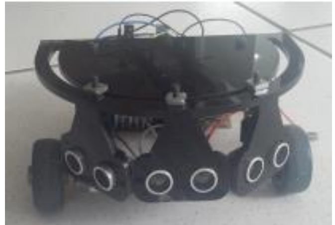
Figure 1: Mechanical structure of the robot.
