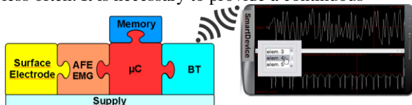
Figure 6: System for NCV (AFE: AnalogFrontend; \mu C: Microcontroller; BT: Bluetooth)
