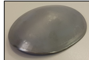
Figure 9: Craniofacial prosthesis made with ISF, applying the design procedure for the anchoring system.
