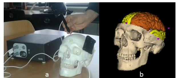
Figure 3: Phantom with attached position tool, surgical pointer and tracking unit (a), and segmented image space (b).
