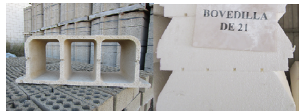
Figure 1. Modeled Materials for lightening elements.
